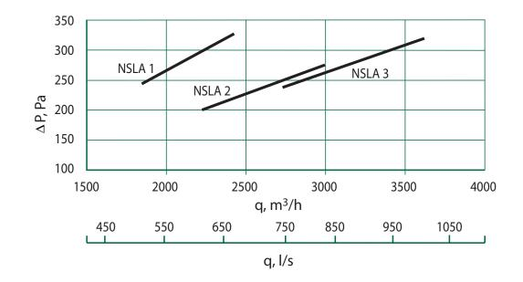
Air flow and design pressure drop for a terminal with a HEPA filter of class H13
