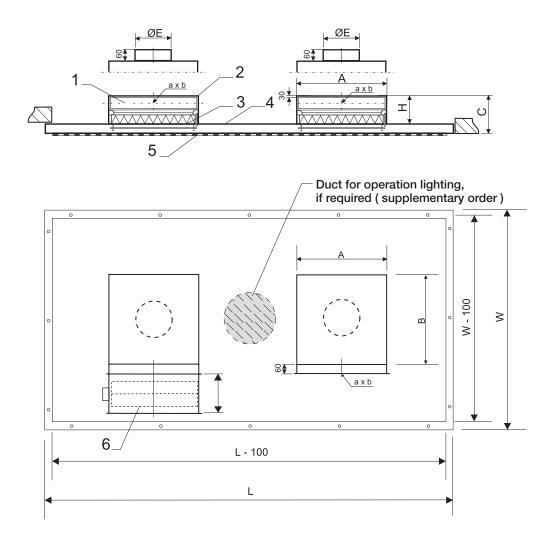
For filters with a height other than 69 mm, the height dimension, H may be different.
